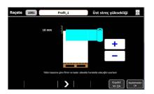
The dimension of stretch exceeding the load can be adjusted.
